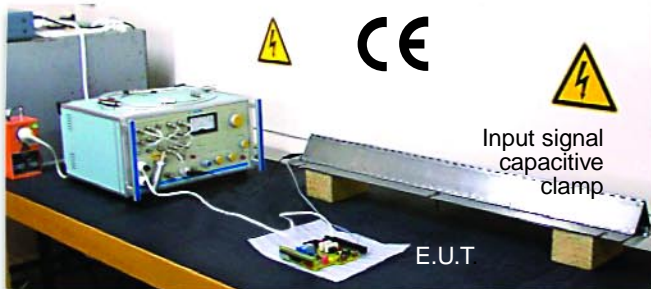
NOISEKEN Burst Testing, Direct and Coupled. Selectable pulse width from 50nS to 1.2µS at 0 to 100Hz with sub nano sec rise time.
