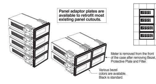
The 48x24mm case is particularly suitable for mounting in mosaic panels or insulative panels up to 2" thick. They can also stack mount, 2 up in existing cutouts for 1/16 DIN (48x48mm) or 4 up in 1/8 DIN (48X96mm).
