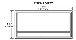
This NEMA Case will fit any existing cutout with dimensions that are between the Snug and Loose Fitting dimensions shown below.
