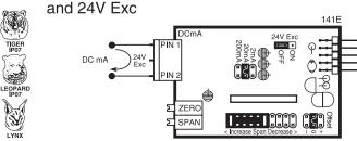
IP01: Process Loop, 4-20mA with 24VDC EXC
