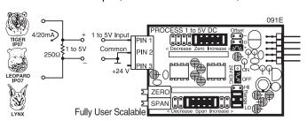
IP07: Universal Process Input 2V/5V/10V/20V/200V/2mA/20mA/Custom
