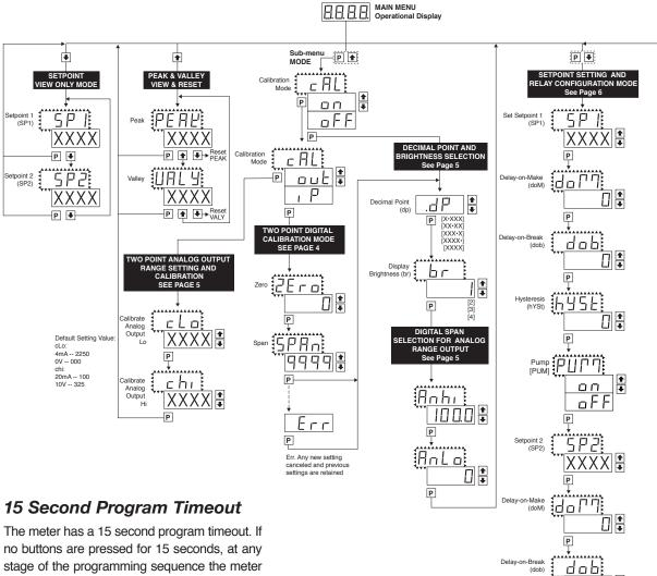
When PUM is selected ON, and SP2 is set at a value higher than SP1, the SP1 relay will operate in a special "pump on pump off" Hysteresis mode. SP2 acts as the upper limit and SP1 acts as the lower limit of the Hysteresis Band.
