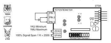
**IR03**: Linear Potentiometer  $1K\Omega$  min
