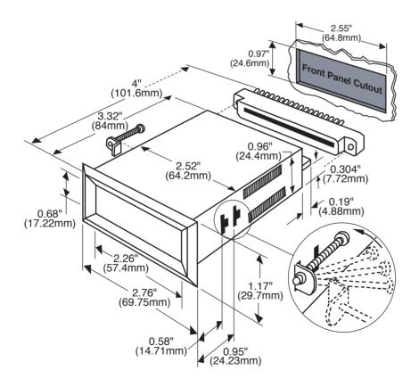
Insert dpm through cutout hole from front of panel. Attach mounting brackets and screws as shown, using second slot when panel thickness is greater than 1/4 inch. Tighten screws against rear of panel.
