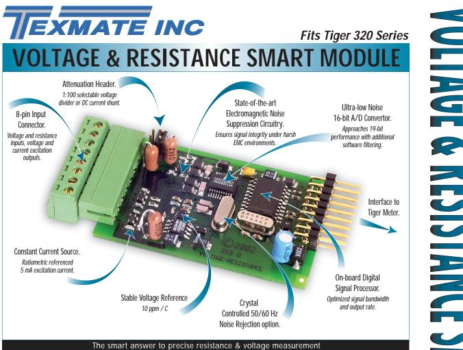
Initially designed to measure copper winding resistance to within fractions of an ohm and the surface temperature using an infrared sensor. When coupled with the Tiger 320 Series operating system this module, and its on-board current and voltage excitation outputs, satisfy OEMs wishing to accurately measure a range of resistance and voltage/current signals.
