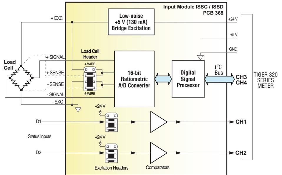
Figure 3 – ISSC / ISSD Signal Flow Diagram
