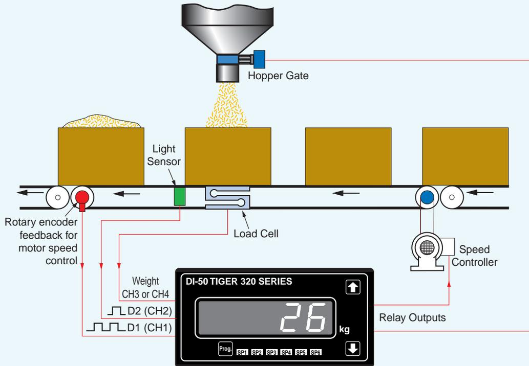
**Figure 5 – Load Cell with Dual Status Inputs**
