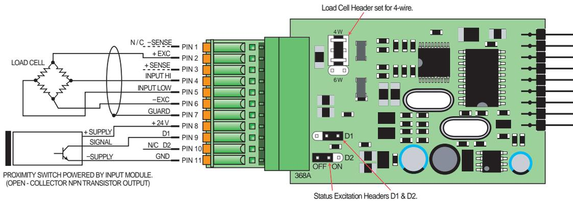
ISSC / ISSD input module showing 4-wire load cell configuration and one status input connected to a proximity switch.
