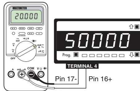
Figure 14 – Multimeter to Meter Connections
