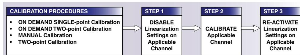
Figure 3 – Linearization Table De-activate/Re-activate Process
