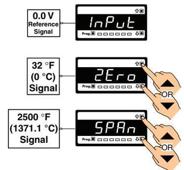
Figure 9 – Thermocouple Calibration
