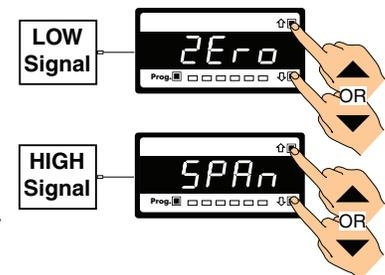
**Figure 8 – Two-point Calibration**
