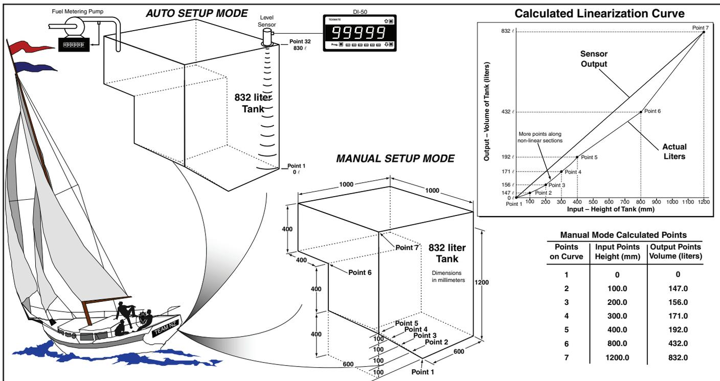
Figure 15 – Example of Manual and Auto Linearization Data
