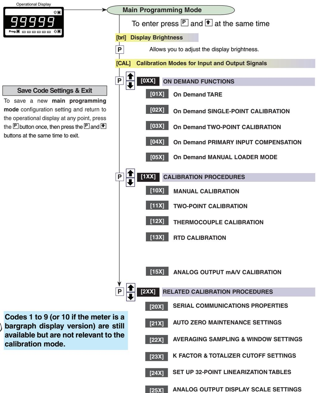
Figure 1 – Calibration Mode Programming Code List
