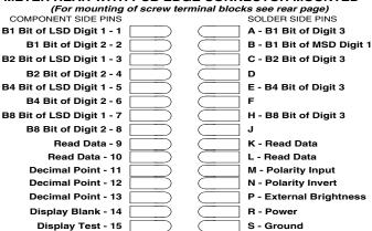
**Pins 1, 3, 5 and 7** are the B1, B2, B4 and B8 bits of the LSD Digit 1 respectively. +5V on these lines corresponds to a High Level (1), and 0V on these lines corresponds to a Lo Level (0).
