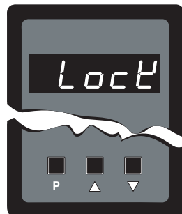
Display Showing [LoCk] Message
