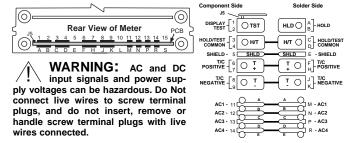
Pins 1 & 2 - Display Test: All numeric display segments will light up when this pin is connected to the H/T Common Pin. A Texmate TB-KIT Screw Terminal Clip can be used to access the Display Test function.
