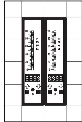
The 96x24mm case is particularly suitable for mounting in mosaic panels or insulative panels up to 2" thick. They can also stack mount, 2 up in existing cut-outs for 1/8 DIN (96x48mm) or 4 up in 1/4 DIN (96x96mm).
