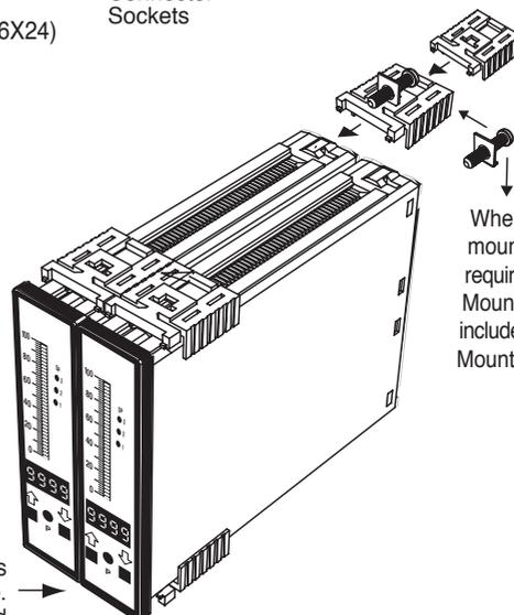
When extra panel mounting tightness is required, optional Screw Mounting Clips are included, which fit on the Mounting Slide Clips.
