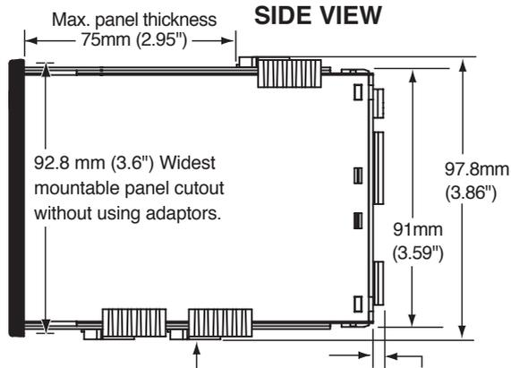
For additional strength, extra Mounting Slide Clips can be ordered and doubled up one behind the other. (P/N: 75-DMT96X24)
