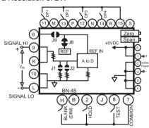
Ratiometric Voltmeter with External Reference To use the BN-45 as a ratiometric voltmeter with an external reference, open J8 and close J9 jumpers. Connect as shown in the diagram.
