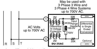
The unique differential input allows safe phase to phase AC line voltage measurements up to 700V AC.
