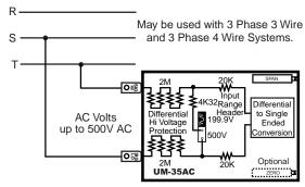
The unique differential input allows safe phase to phase AC line voltage measurements up to 500V AC.
