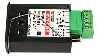
Pin 1 = +5VDC Pin 2 = Ground Pin 3 = Signal LOW Pin 4 = Signal HIGH Pin 5 = DIM (Dimming pot between Pin5 &3)
