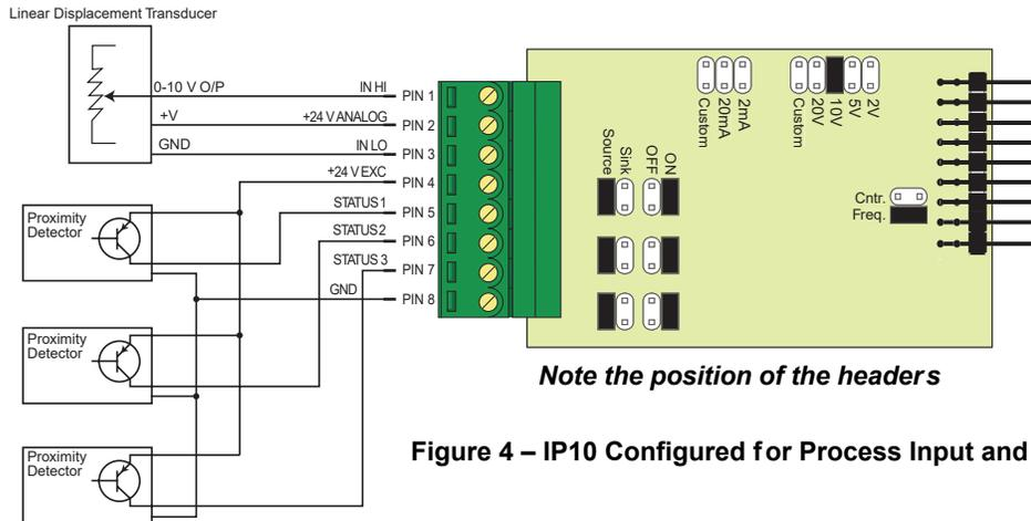
Figure 4 – IP10 Configured for Process Input and Three Status Inputs
