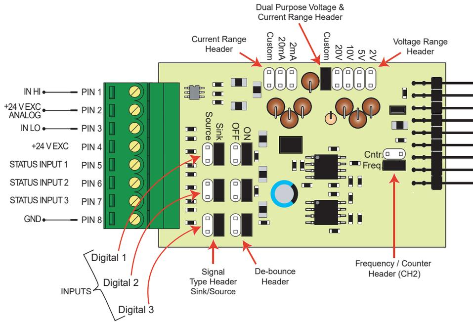
**Figure 1 – IP10 Process / Triple Status Input Module**
