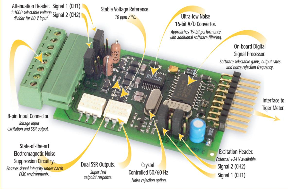
The answer to accurate voltage measurements and switched relay outputs.
