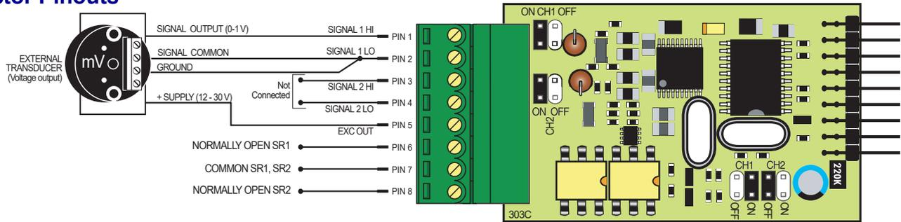
The diagram shows an external transducer requiring external excitation wired to input module ISD3 or ISD4 through signal 1.
