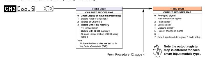
To select channel 4, enter Code 6 and select the required post processing settings for CH4 in the 1st digit and the required register map settings in the 3rd digit.
