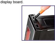
To open meter, insert a flat head screwdriver or similar instrument in both slots on the side of the cover and pry open. The UM-Series meters slide out from the front of the case as a complete assembly.
