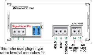
screw terminal connectors for all connections.
