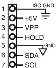
Internal header pins 1, 2, 3, 6, and 7 are for factory settings only. Not for external use!
