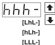
When there are more than two display selections they are shown in brackets below the first display and are also selectable by pressing and releasing the [↑] or [↓] buttons.
