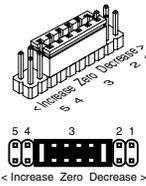
When this header is provided, it works in conjunction with the ZERO OFFSET RANGE Header, and expands the ZERO pot's offset capability into five equal negative steps or five equal positive steps. This enables virtually any degree of input signal offset required to display any desired engineering unit of measure.
