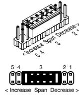
This unique five-position header expands the adjustment range of the SPAN pot into five equal 20% steps, across 100% of the input Signal Span. Any input Signal Span can then be precisely scaled down to provide any required Digital Display span from 1999 counts to 001 (one count).
