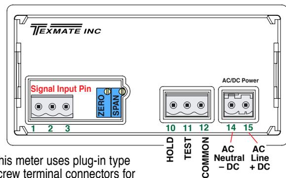
This meter uses plug-in type screw terminal connectors for all connections.
