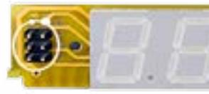
Decimal selection is made by moving the jumper to the indicated position on the header for the decimal required on the front of the display board.
