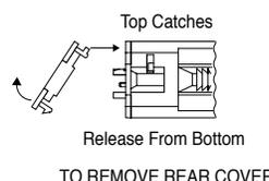
To open back panel, insert a flat screwdriver or similar instrument in both slots on the top of the case and pry open. The BX-Series meters slide out from the rear of the case as a complete assembly.
