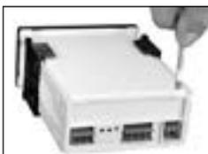
To open back panel, insert a flat screwdriver or similar instrument in both slots on the top of the case and pry open. The DX-Series meters slide out from the rear of the case as a complete assembly.
