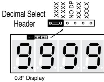
Decimal selection is made by moving the jumper to the indicated position on the header for the decimal required on the front of the display board.
