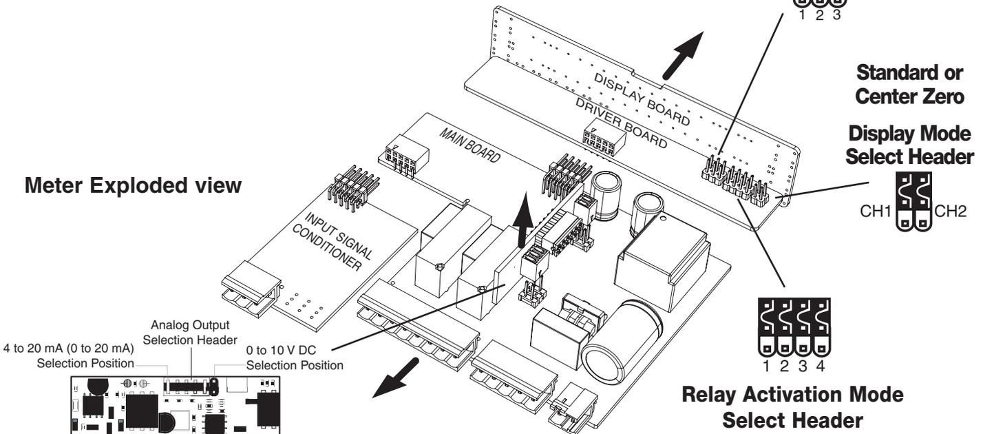
Optional 16 Bit Isolated Analog Output Module
