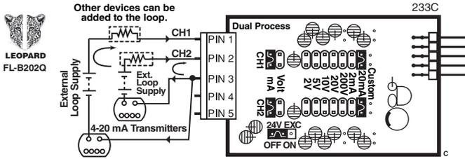
**IDP4 with 4-20 mA Connection and External Setpoint option - excitation provided by the meter**
