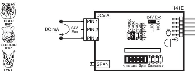
**IDP4 with Dual Channel DC mA, 2 mA/20 mA/Cust Connection (2 mA DC range shown)**
