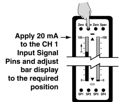
In the Dual input mode, the procedure for calibrating CH2 is the same, except that the input signal is applied to the CH2 input pins and adjustments are made with the CH2 ZERO and CH2 SPAN buttons.
