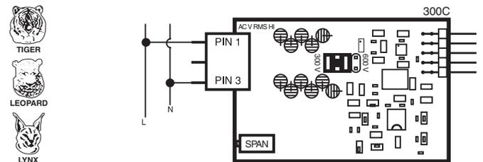
**IA02:** AC Volts Scaled RMS, 200mV/2V/20V AC
