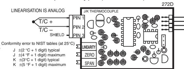
**Dual input modules, and those modules exclusively compatible with the Leopard or Tiger Families, do not have zero and span adjustments. These modules are scaled and calibrated using the internal software functions of each individual meter.**
