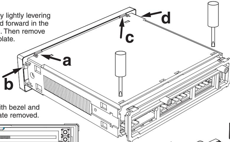
Front view with bezel and scale faceplate removed.
