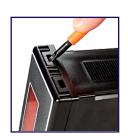
To open meter, insert a flat head screwdriver or similar instrument in both slots on the side of the cover and pry open. The UM-Series meters slide out from the front of the case as a complete assembly.
