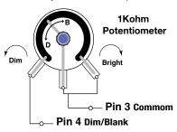
**Hold Reading:** When Pin 5 (Hold) is connected to the Common Pin 3, the meter will freeze the reading while A/D conversions continue. The display will not be updated until the Hold Pin and Common pins are disconnected.
