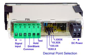
**Display Test:** All numeric display segments will light up when Test Pin 6 is connected to Common Pin 3.
