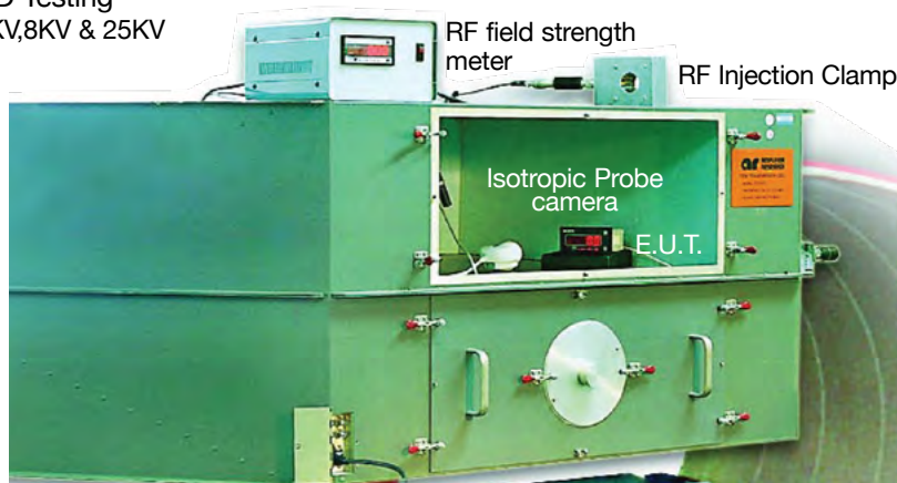
Laboratory TEM Cell for testing RF Immunity and Emissions
