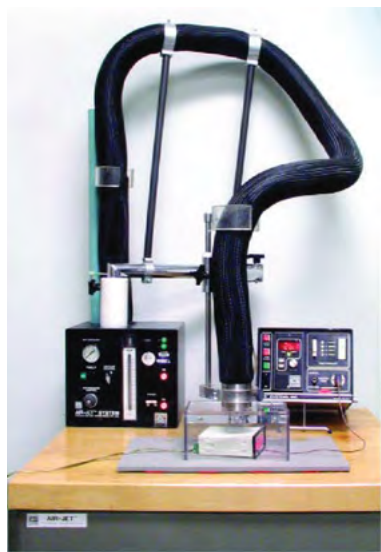
Extreme Temperature Cycling Temperature testing from -40°C to +70°C in 14 seconds
