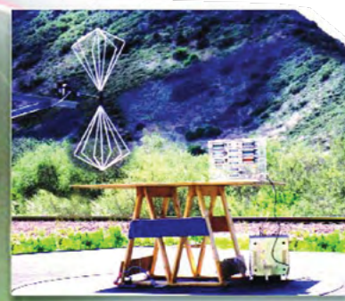
Open Air EMI Emission Testing to CSPP 22
