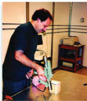
ESD Testing ±2KV,4KV,8KV & 25KV
