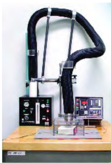
Extreme Temperature Cycling Temperature testing from -40°C to +70°C in 14 seconds
