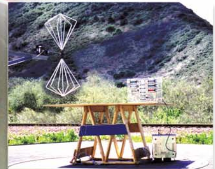
Open Air EMI Emission Testing to CSPR 22
