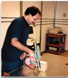
ESD Testing ±2KV, 4KV, 8KV & 25KV
