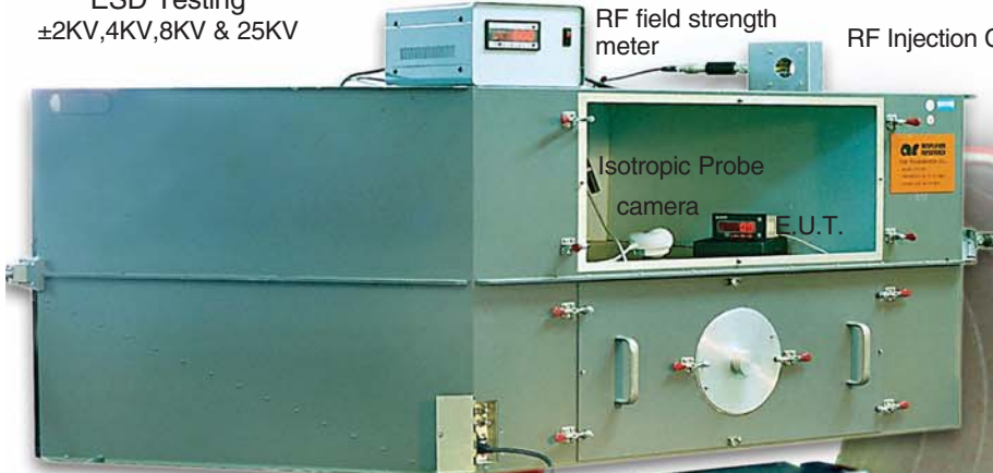
Laboratory TEM Cell for testing RF Immunity and Emissions
