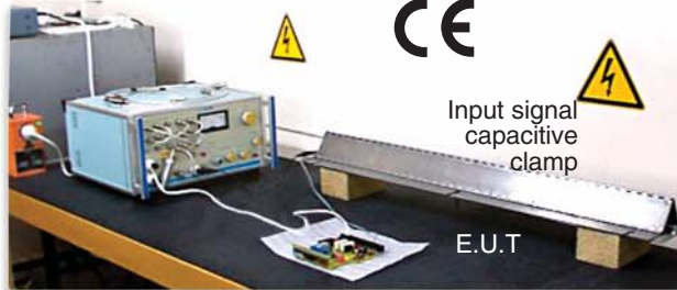
NOISEKEN Burst Testing, Direct and Coupled. Selectable pulse width from 50nS to 1.2µS at 0 to 100Hz with sub nano sec rise time.
