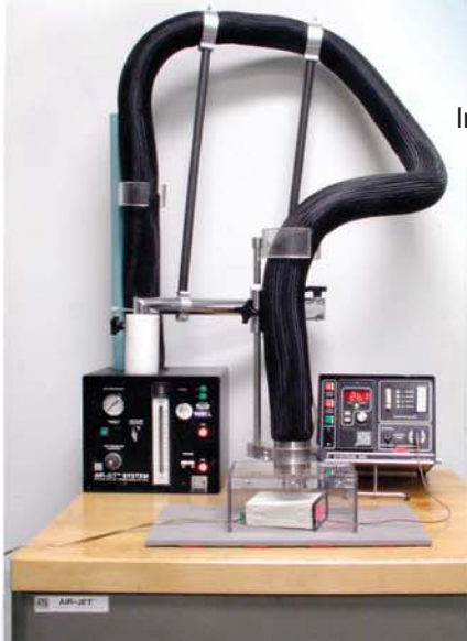
Extreme Temperature Cycling Temperature testing from -40°C to +70°C in 14 seconds
