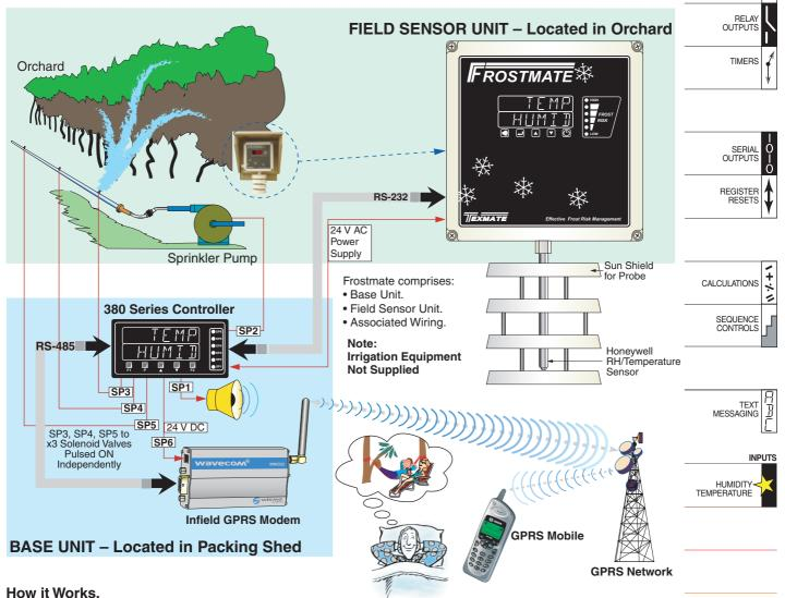
The system consists of two boxed units. The field unit contains a temperature and relative humidity probe connected to a Tiger 320 Series controller and is based in the orchard. Both temperature and humidity are displayed at the same on the dual time display. Annunciators display the frost risk in six levels ranging from low to high.
