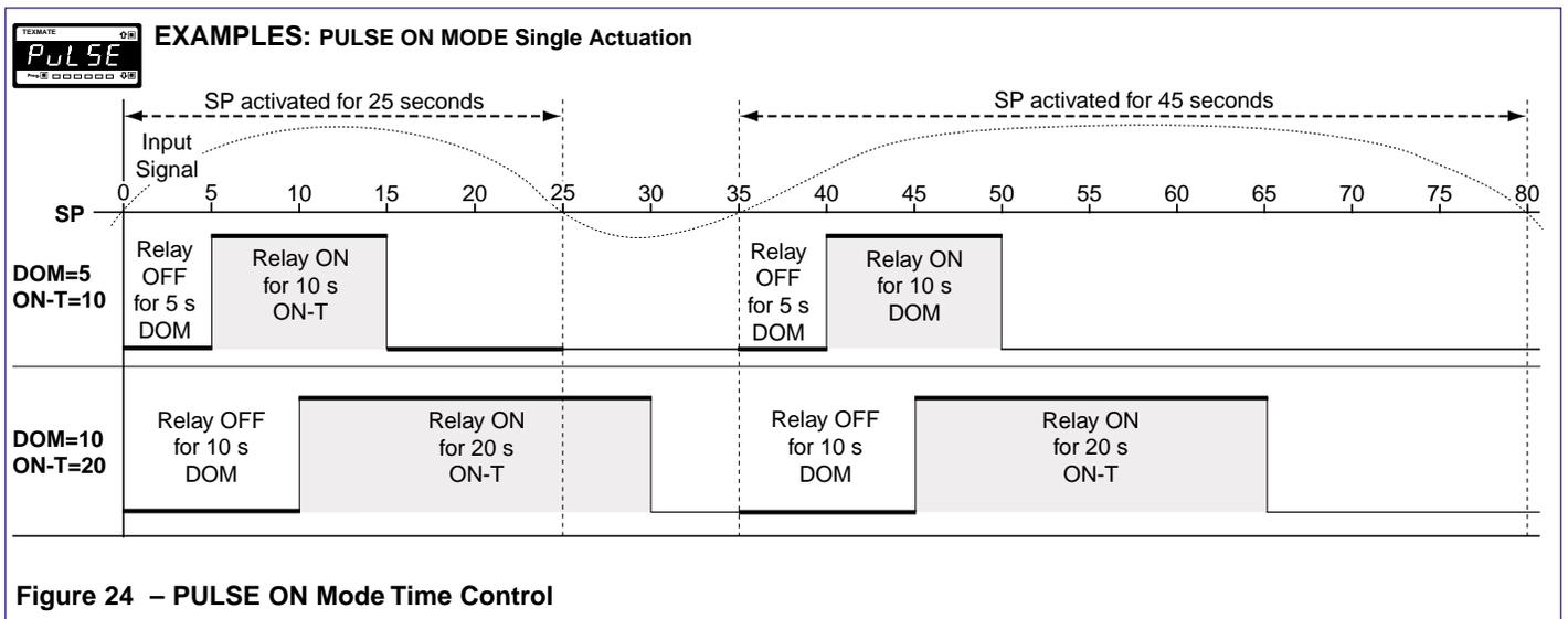
Figure 24 – PULSE ON Mode Time Control
