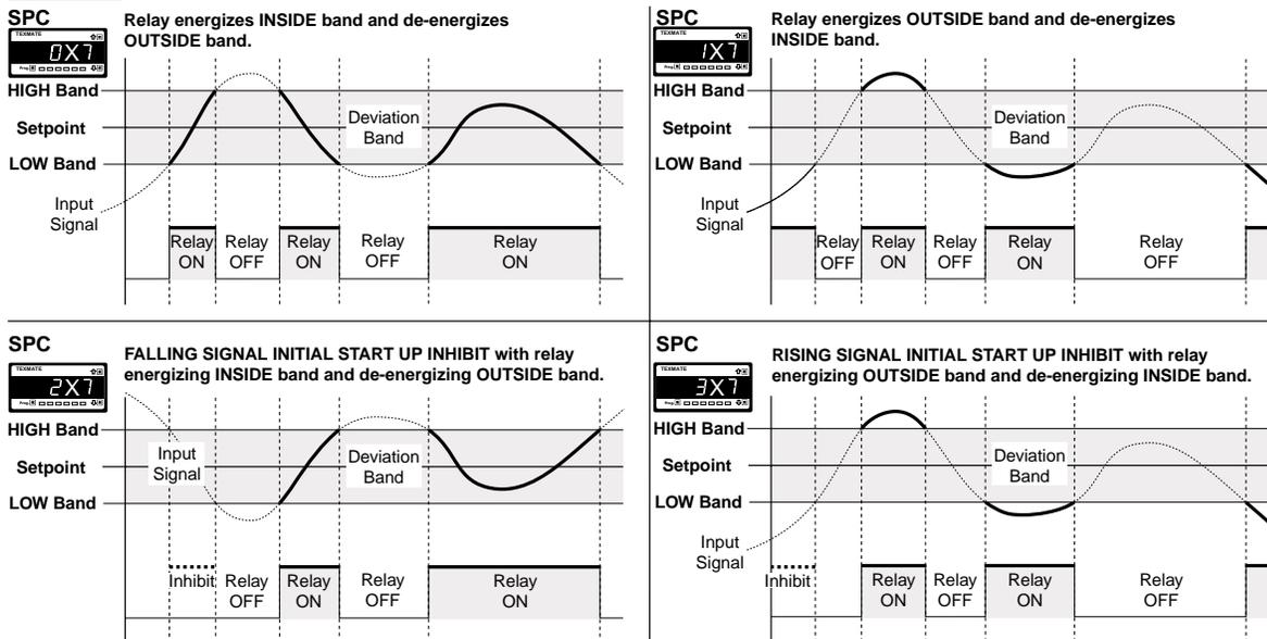
**Figure 14 – Example 2: Relay energize functions with deviation**
