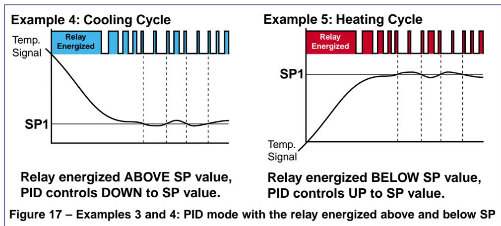
Figure 17 – Examples 3 and 4: PID mode with the relay energized above and below SP
