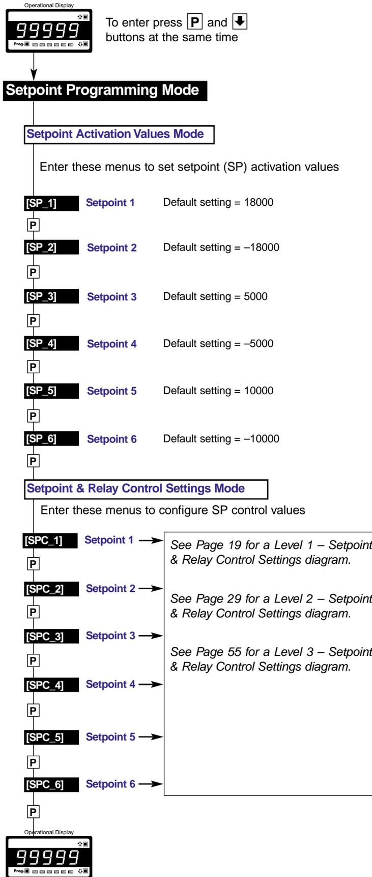
Figure 3 – Setpoint Programming Mode Logic Diagram
