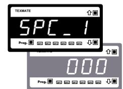
Enter the Setpoint and Relay Control Functions Mode and program the control settings for each setpoint relay in turn (SPC\_1 thru SPC\_6)
