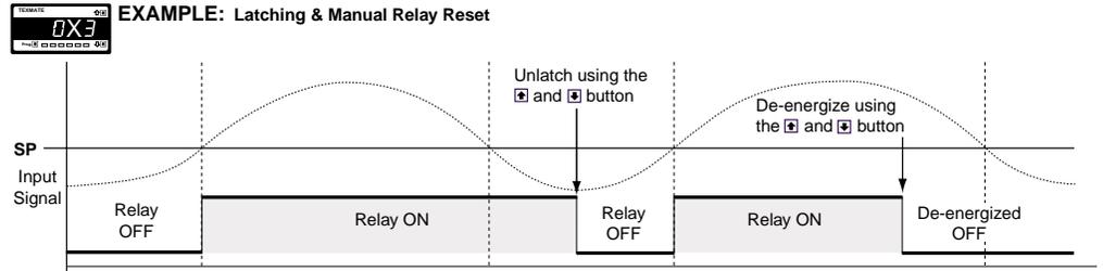
Figure 8 – Latching & Manual Relay Reset
