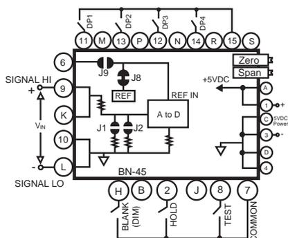
Ratiometric Voltmeter with External Reference
