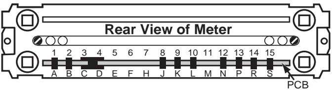
**METER REAR WITH PCB EDGE CONNECTOR MOUNTED**
