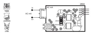
IAO4: AC Amps Scaled RMS, 1 Amp AC IAO5: AC Amps Scaled RMS, 5 Amp AC
