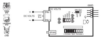
IDO2: DC Millivolts, 20/50/100/200mV DC w/24V DC Exc
