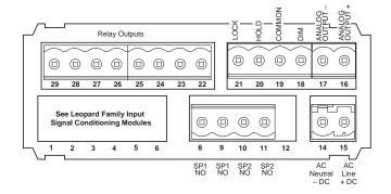
Auto-sensing AC/DC power supply. For voltages between 85-265 V AC / 95-370 V DC (PS1) or 18-48 V AC / 10-72 V DC (PS2). Standard plug-in screw terminal connectors provided by Texmate:
