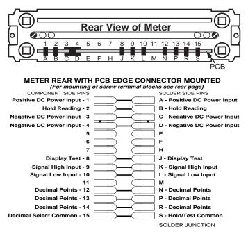
**Pins 1 & A - Positive 5V DC Power Input:** These pins are internally connected together. The positive end of the DC power is connected to these pins. The standard BN-45 meter is designed to be powered from a 5VDC power supply. Isolated power supplies options for 12V, 15V or 24V DC are available using the model BN-45I.
