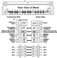
WARNING: AC and DC input signals and power supply voltages can be hazardous. Do Not connect live wires to screw terminal plugs, and do not insert, remove or handle screw terminal plugs or internal jumper clips with live wires connected to the meter.
