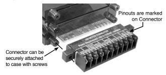
A standard 30-pin edge card connector can be used to connect the DD-40VHz. As an alternative, however Texmate has designed an extremely easy-to-use connector called the Push-On™ connector. This exclusive connector design combines an edge card connector and screw terminal blocks into one piece. To order, use part number DD-PUSH/DD.
