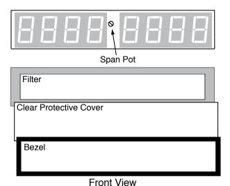
The DD-40VHz is calibrated at the factory with a precision AC voltage source. A calibrator of 0.05% accuracy is required to completely check the operation of the DD-40VHz meter.
