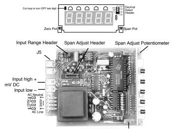
**UM-45MV** Zero Adjust Potentiometer
