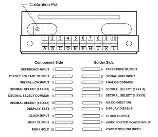
CAUTION: This meter employs high impedance CMOS inputs. Although internal protection has been provided for several hundred volt overloads, the meter will be destroyed if subjected to the high kilovolts of static discharge that can be produced in low humidity environments. Always handle the meter with ground protection.
