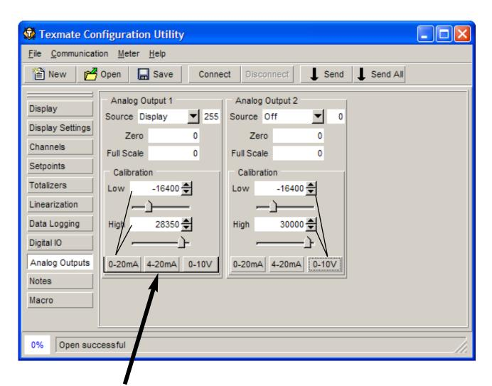
Press button for default calibration values. Exact calibration has to be done for each board separately.
