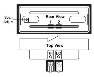
**Pin 1 - Input Hi:** This is the signal high input to the meter. Voltages from ±3.5V to 199.9V DC may be measured.
