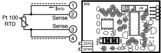
Sense input leads should be joined to the IRTD leads as close as possible to the sensor element because, on 2 wire RTDs, the single lead length resistance from the sensor to these joints will produce uncompensatable errors. Excitation is 1mA. Up to 50 resistance in each lead can be compensated.
