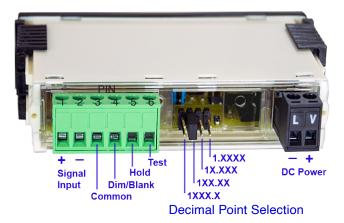
**Display Test:** All numeric display segments will light up when Display Test Pin 6 is connected to Common Pin 3.
