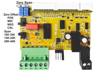
Zero offset and Span header/jumpers are used for display scaling. Scaling defaults to 00.00 - 100.00(%); contact Texmate for your custome scaling needs.
